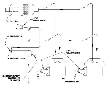
Figure 4: Vertical Phillips Dry Oil Separator Note that flow is reversed with drain at inlet end of separator.
