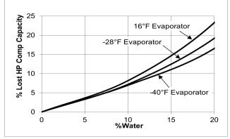
Chart assumes increased suction temperature due to water and 2.4% lost compressor capacity per  $^{\circ}$ F.
