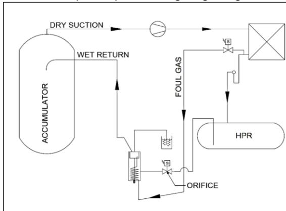
**Figure 8: HPL Feed System Installation Example**
