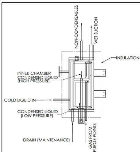
**Figure 2: Basic flow through the Purger**
