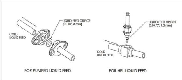
**Figure 10: Temporarily Remove Orifices before Welding**
