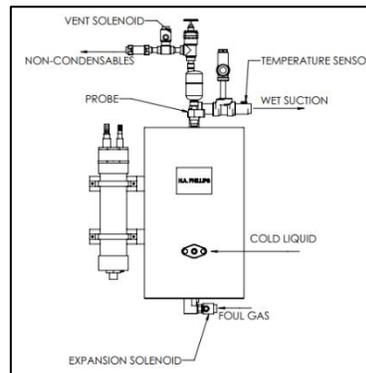
**Figure 3: Purger Control Components**
