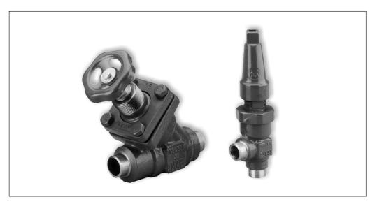
SVA are angle-way and straight-way stop valves. The valves have internal backseating enabling the spindle seal to be replaced with the valve still under pressure. They are furthermore carefully designed to give favourable flow conditions. Easy to disassemble for inspection and repair, if
