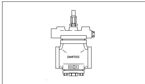
Code number includes: PM 3 valve with flange gaskets and bolts (but without flanges)
