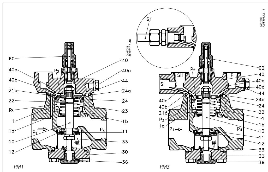
The PM main valve is a pilot operated valve whose function is determined by the pilot valve used. The main valve with pilot valve(s) controls refrigerant flow by modulation or on/off in accordance with the pilot valve or main valve status.
