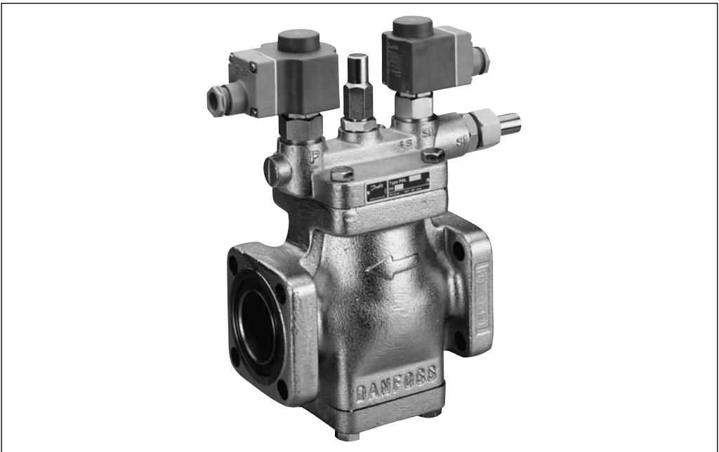
PMLX are 2-step servo-operated main valves with screwed-on pilot solenoid valves. PMLX valves use an external pressure source for opening (which means that no differential pressure across the PMLX valve is required).
