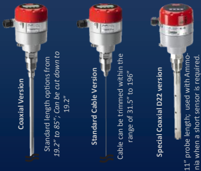
AKS 4100U Liquid Level 4-20 mA; Coaxial or Cable Versions
